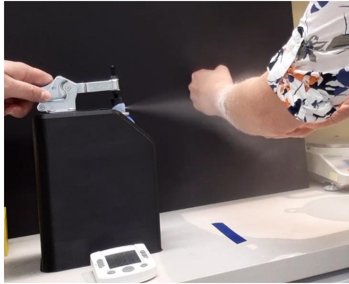
Figure 3. The actuator device. The calibrated actuator device dispersing a jet-spray of sunscreen onto an arm 10cm away from the bottle.
