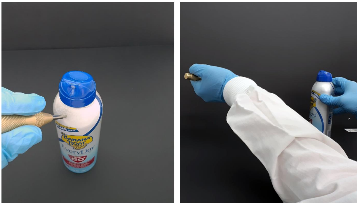
Figure 2. Degassing of Aerosol Sunscreens. Left panel, a pin hole is made to the pressurized can for the propellant gas to escape. Right panel, the pin hole allows propellant gas to escape and the liquid sunscreen remains in the container.
