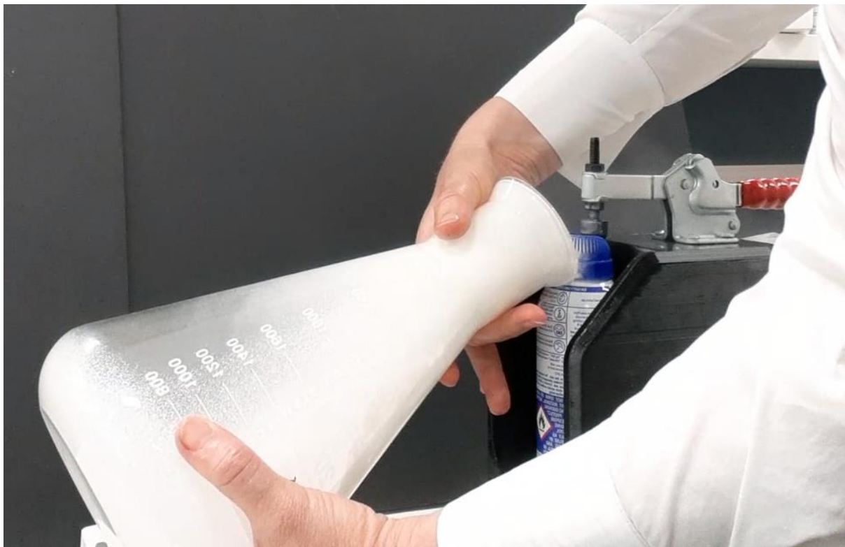
Figure 5. The experiment to determine the length of time each product can be sprayed. The actuator device dispersed sunscreen from the aerosol sunscreen product into a large collection flask until the sunscreen bottle was empty.
