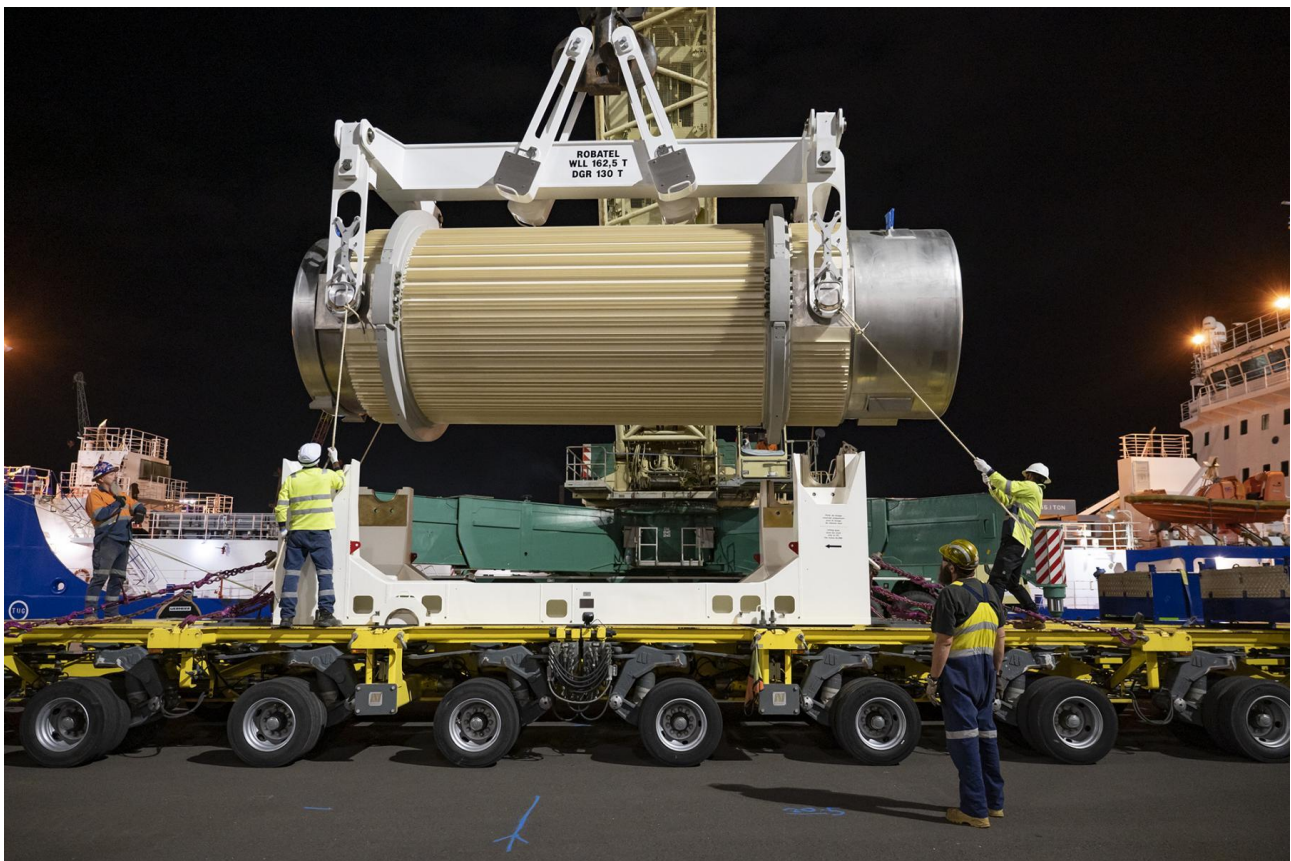
Figure 2: TN-81 transport and storage package carrying reprocessed spent fuel waste residues being prepared for road transport to ANSTO (2022).
