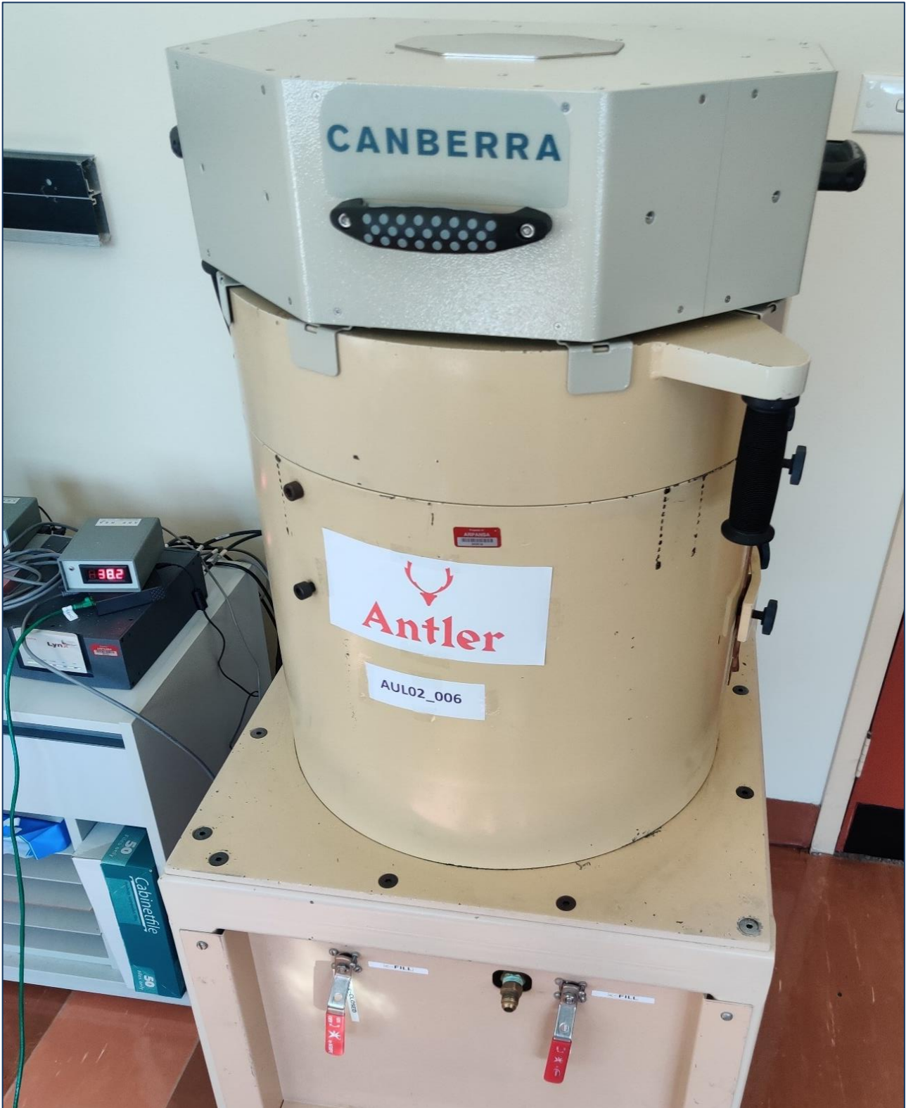
Figure 1: Image of CosmicGuard veto system installed on CRL Antler detector system
